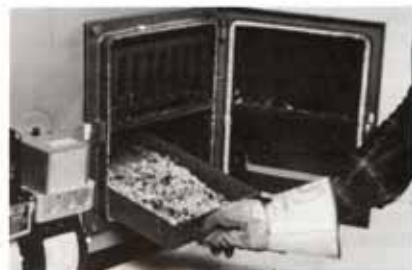
Ash scoop is used for emptying. Ashes should be removed before they touch grates and restrict airflow.
