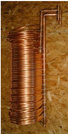
Space heat exchanger
